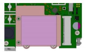
Install module to the miniPCle slot and secure with previously removed screws. Tightening torque 0,3 Nm.
