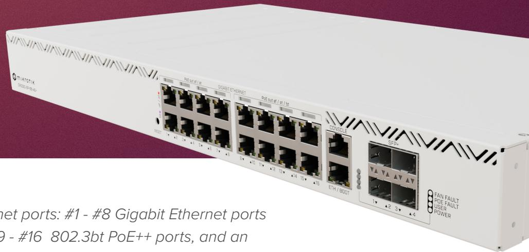
*There are 17 Gigabit Ethernet ports: #1 - #8 Gigabit Ethernet ports with 802.3af/at PoE-out, #9 - #16 802.3bt PoE++ ports, and an extra Gigabit Ethernet port for management purposes. There's also a console port, and four 10G SFP+ fiber ports for uplink.*
